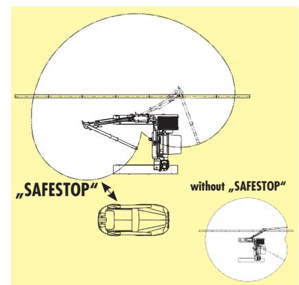
\* With more powerful lifting hose unit, proper suction plate etc. and platform for counterweight TM-GGP upgradeable to 200 kg lifting capacity when fully extended and up to 250 kg at reduced outreach of 500 mm.
